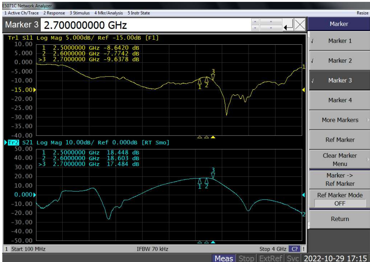
Figure 4: Network analyzer output, S11 and S21
