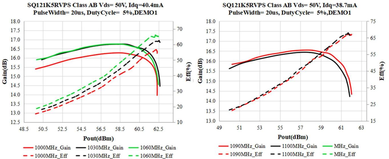
Figure 2. Power Gain and Drain Efficiency as Function of Pulse Output Power (1030-1090MHz)
