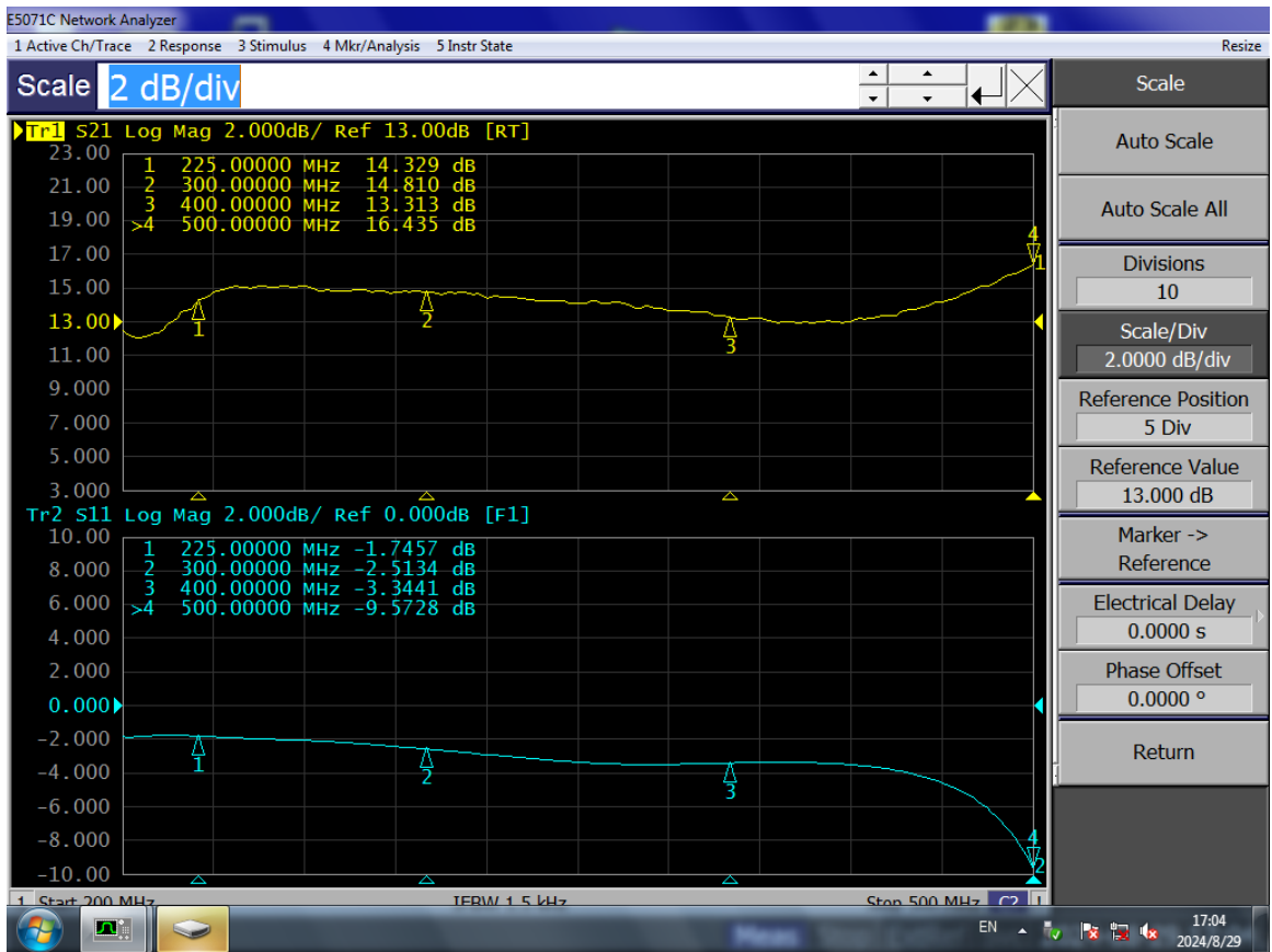
Figure 4: Network analyzer output, S11 (Vds=50V, Idq=700mA, Vgs=3.45V)
