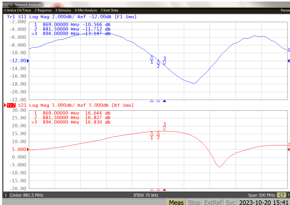
Figure 5. Network analyzer output S11/S21
