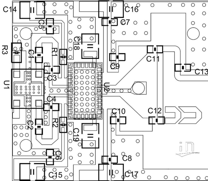
Figure 2. Test Circuit Component Layout
