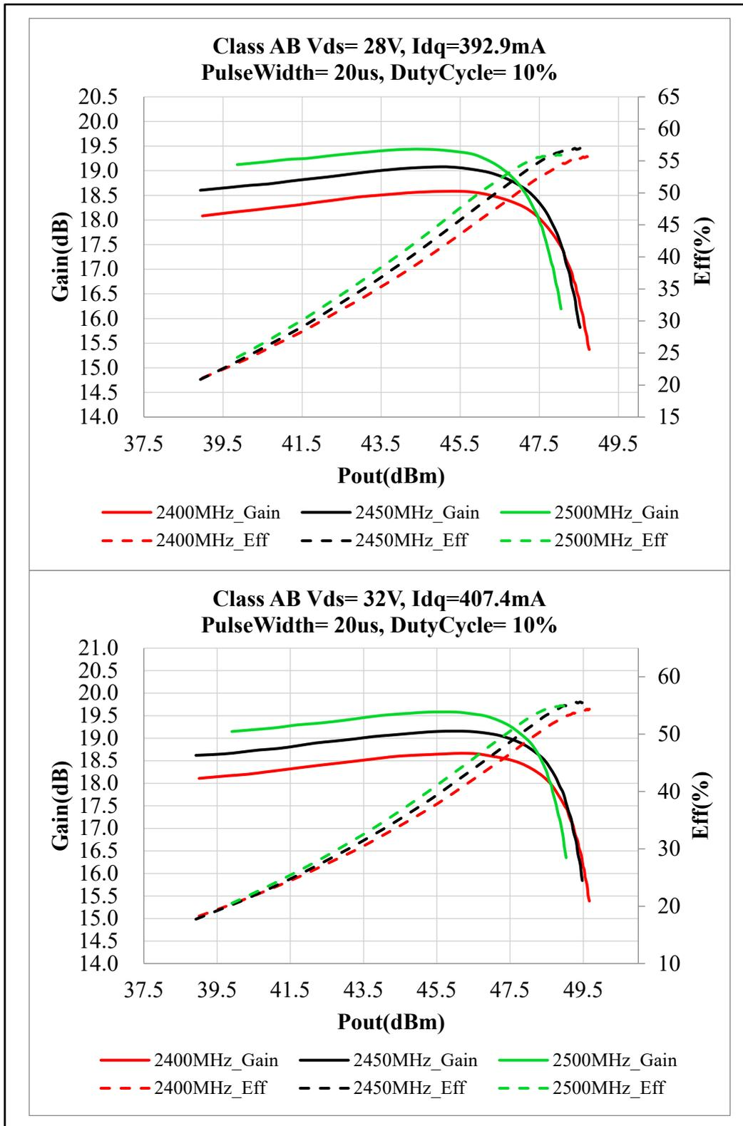
Figure 2. Power Gain and Drain Efficiency as Function of Pulse Output Power
