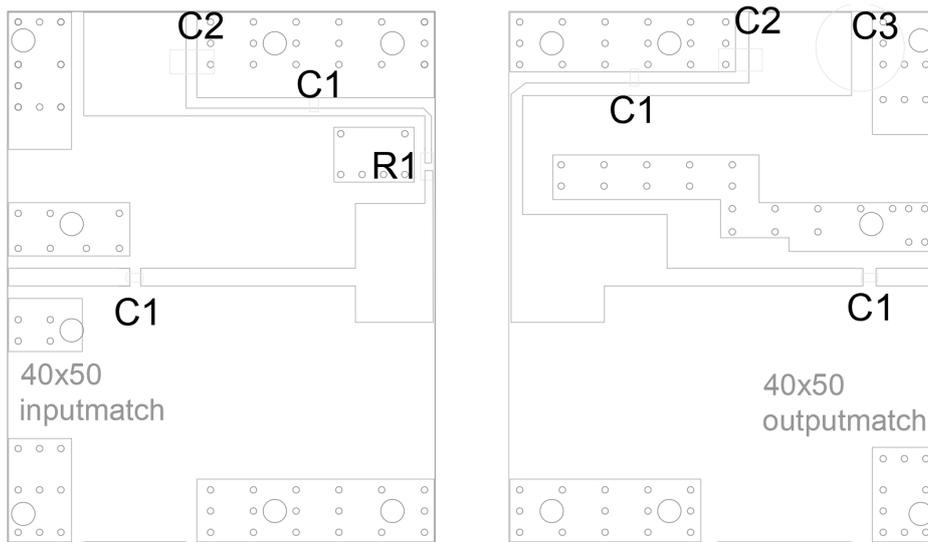
Figure 1. Test Circuit Component Layout (2400MHz~2500MHz)
