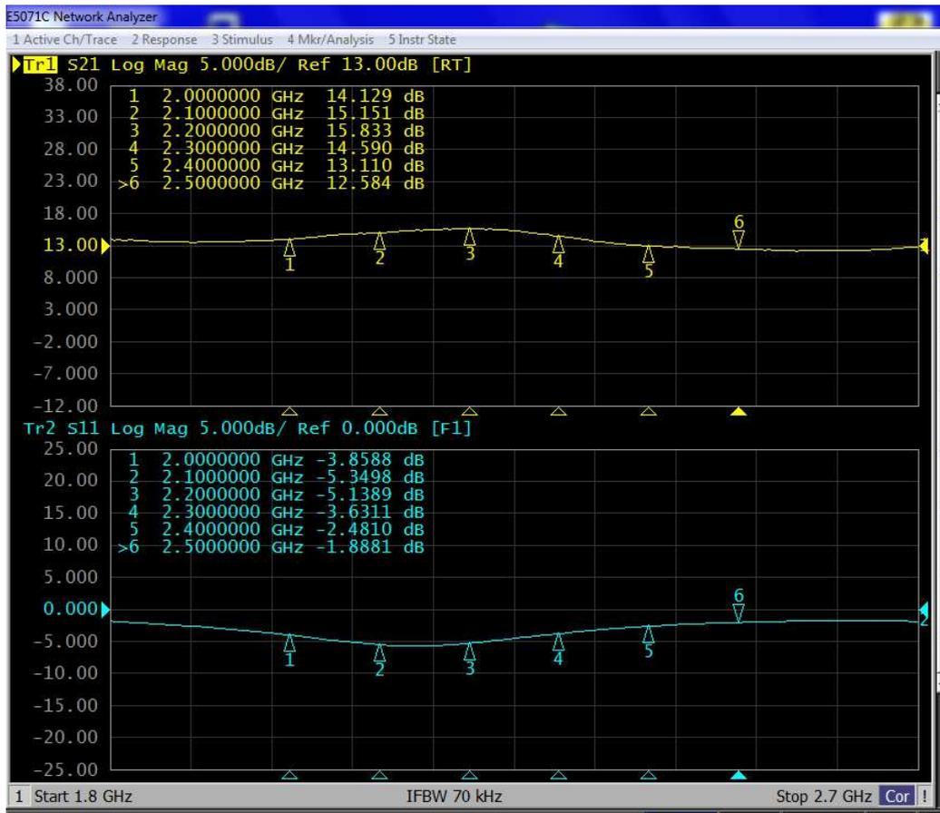
Figure 1. Network analyzer output S11/S21, Idq=1A, Vds=28V
