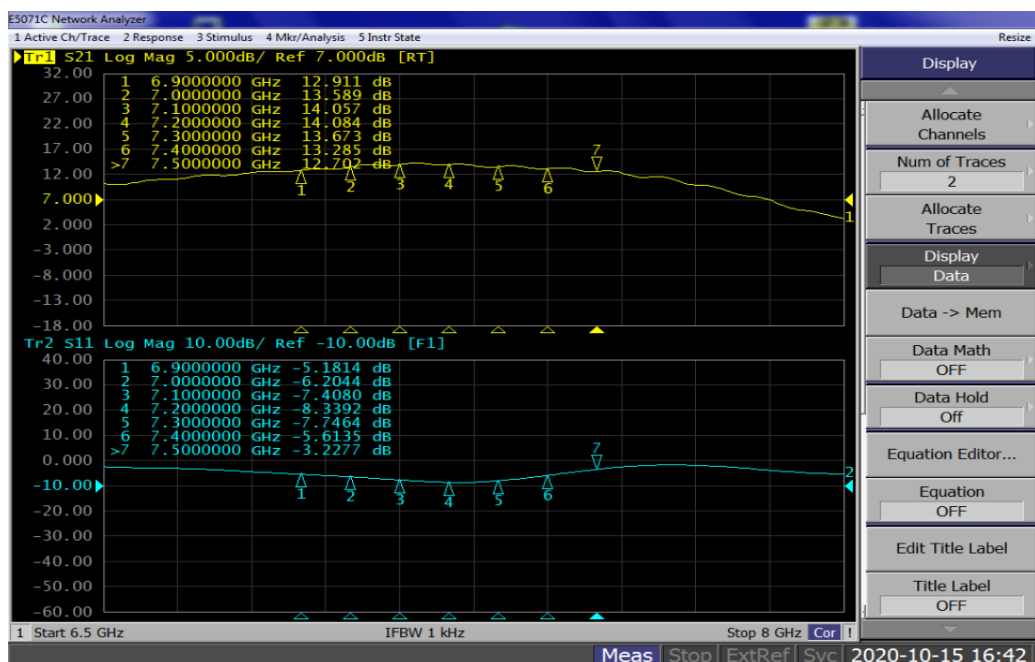
Figure 2. Network Analyzer S11/S21 output ( V_{ds}=28V, V_{gs}=-2.46V, I_{dq}=20mA , Input Power =0dBm)
