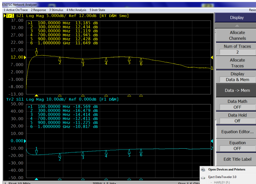
Figure 1. Network analyzer output S11/S21 (Pin=0dBm) @50V
