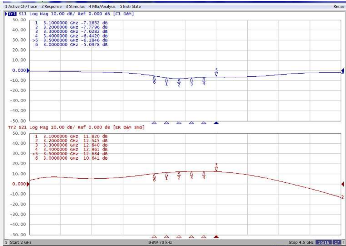
Figure 4. Network analyzer output S11/S21
