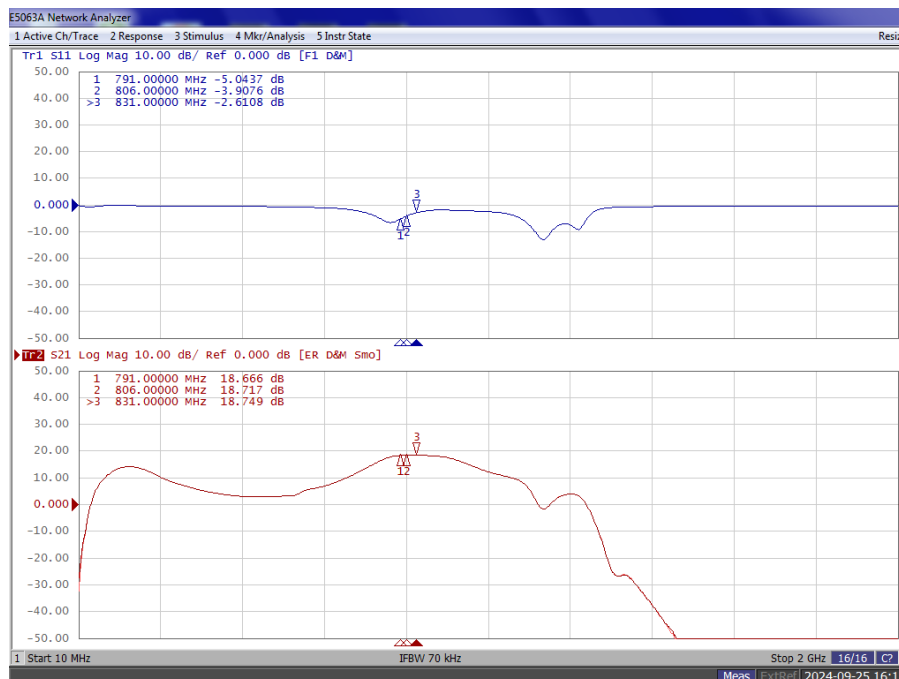
Figure 3: Network analyzer output, S11 and S21
