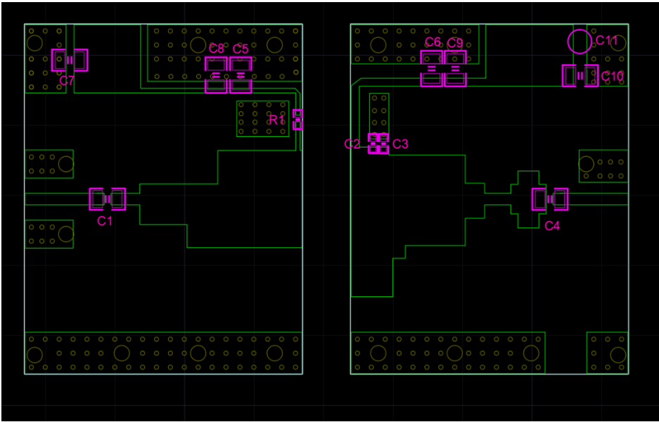
Reference Circuit of Test Fixture Assembly Diagram (Layout file upon request)
