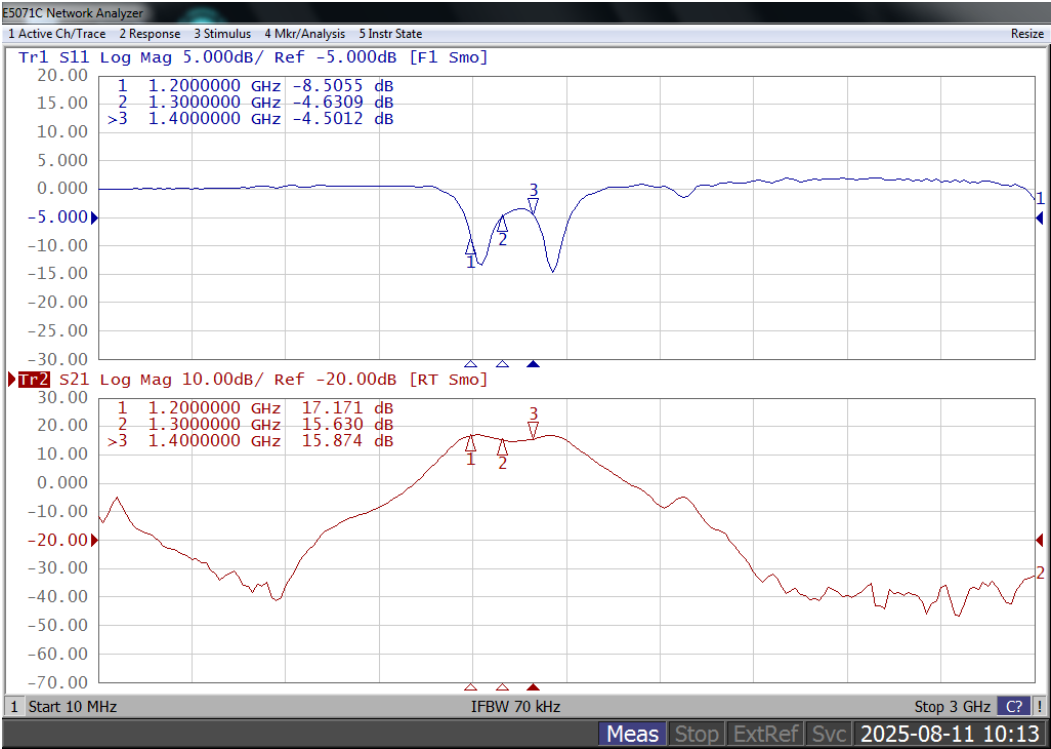
Figure 3: Network analyzer S11 and S21
