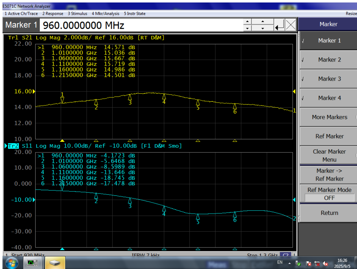
Figure 2: Network analyzer output S21/S11 (Vds=50V, Idq=600mA)
