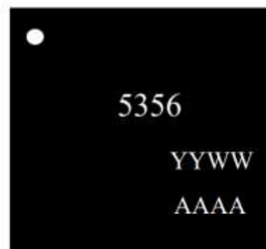
20-pin 4.0 mm x 4.0 mm x 0.9 mm QFN package
