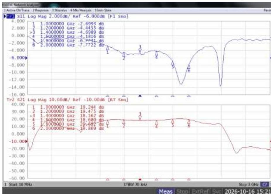
Figure 2: Network analyzer output, S11 and S21 ( V_{\text{DS}} = 50\text{V} V_{\text{GS}} = -3.4\text{V} I_{\text{DQ}} = 250\text{mA} )
