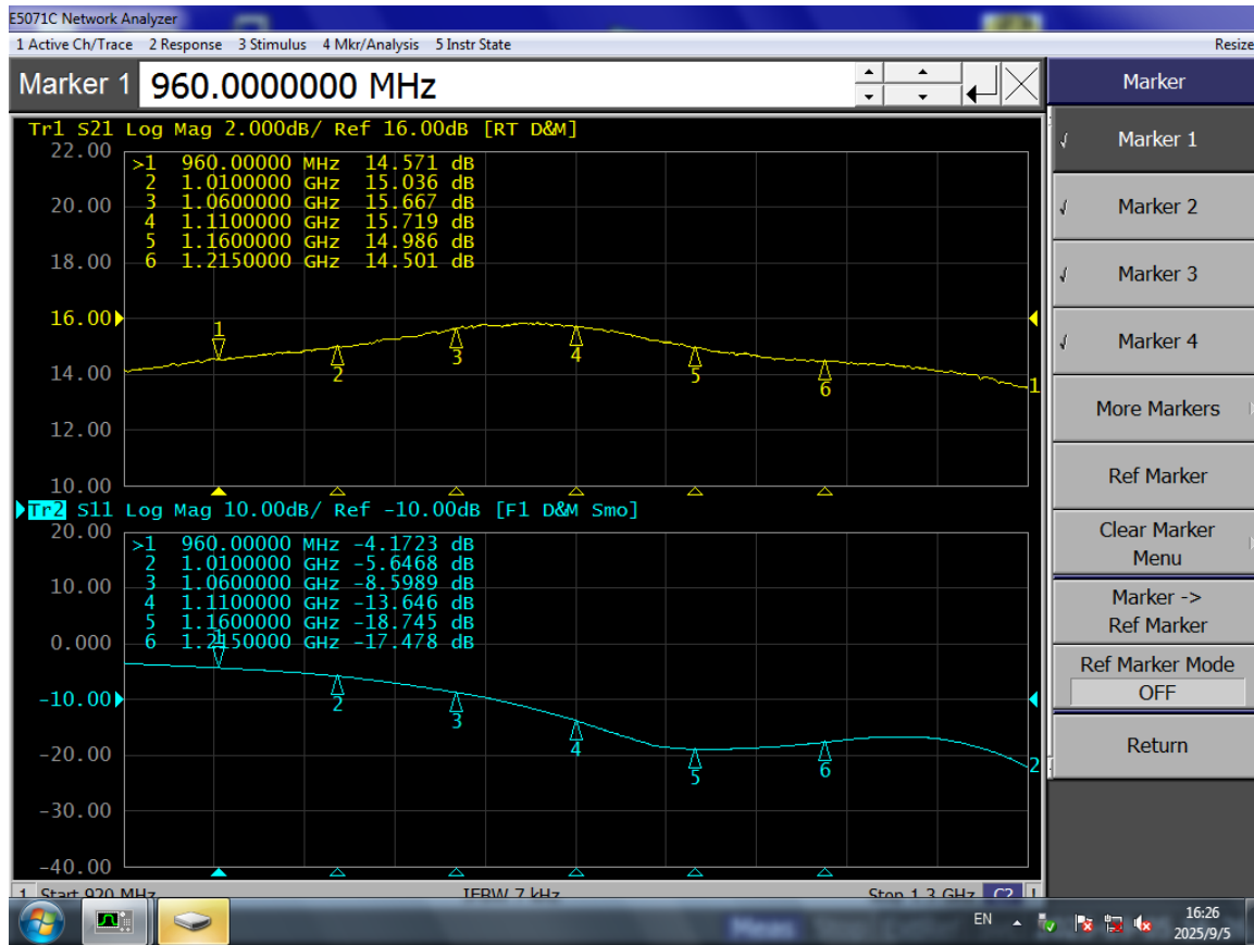
Figure 2: Network analyzer output S21/S11 (Vds=50V, Idq=600mA)
