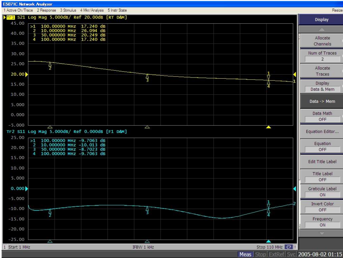
Figure 2: Network analyzer output S21/S11 (Vds=50V, Idq=1000mA)
