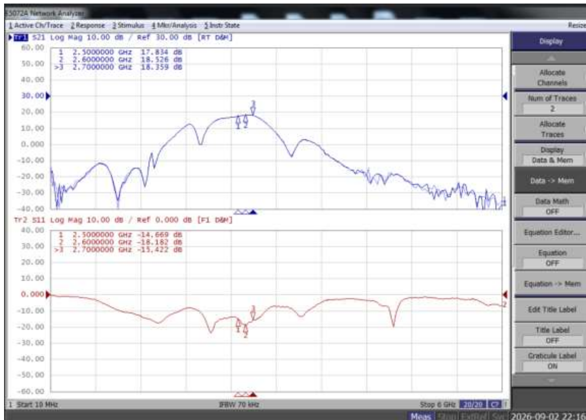
Figure 4: Network analyzer output, S11 and S21 (2.5-2.7GHz Doherty)
