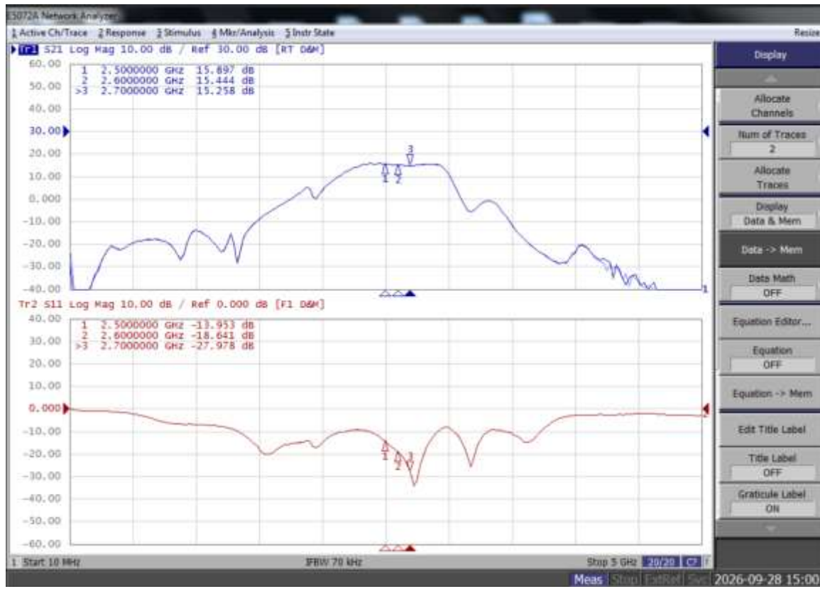
Figure 5: Network analyzer output, S11 and S21
